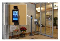
Face recognition system with a thermography camera
