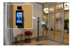
Face recognition system with a thermography camera
