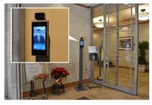
Face recognition system with a thermography camera
